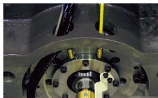
Cooling system of the ball screw bracket
